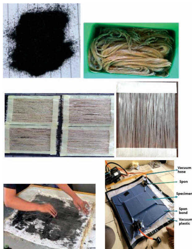
Figure 1: a) Bamboo-activated carbon nanofiller powder; b) abaca fiber soaking; c) dried abaca fiber arranging; d) E-glass fiber arranging; e) hand lay-up composite lamination; f) vacuum bagging composite lamination
